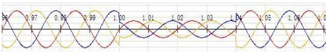
Figure 4.2.2.3.9.1 Waveform Screenshot of Voltage Swell
